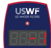
At any point during this sequence, the audible chirp or alarm can be deferred for seven days by holding the controller button down for a period of five seconds. The number of deferrals used will be displayed as below. Once the deferral expires, the alarm will sound once again. The deferral can be repeated up to three times. **PLEASE NOTE:** At any point after lamp expiration, the water disinfection rate will be compromised.
