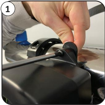
1 Remove **ONLY** the top mounting bolt from controller.
