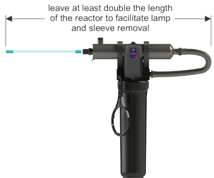
Figure 12. Lamp Removal Spacing
